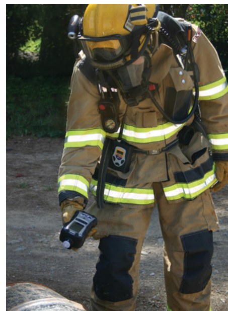
MultiRAE Pro with RAELink3 Mesh used for screening potentially hazardous drums
