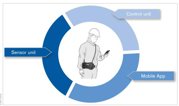
The Dräger X-pid® 9500 consists of three elements: You control the sensor unit via the control unit and the pre-installed mobile app. The sensor unit can be worn around the neck, keeping one hand free.
